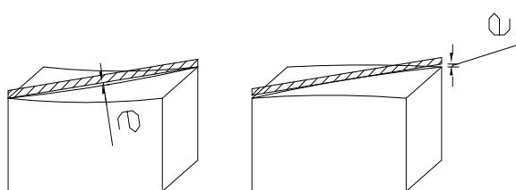
1. Installing face: put the steel square (side length 500mm) on the surface of the product in the diagonal direction. Fine machined depth:  $e \leq 1\text{mm}$ ; Rough machined depth:  $e \leq 2\text{mm}$
