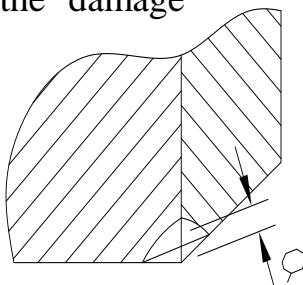
damage  $a \leq 30\text{mm}$  and two such defects in one block are unaccepted.
